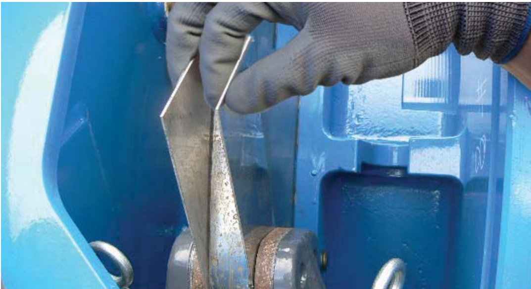
Figure 4: Adjusting the Air Gap Using Two \frac{1}{16} " Shims
